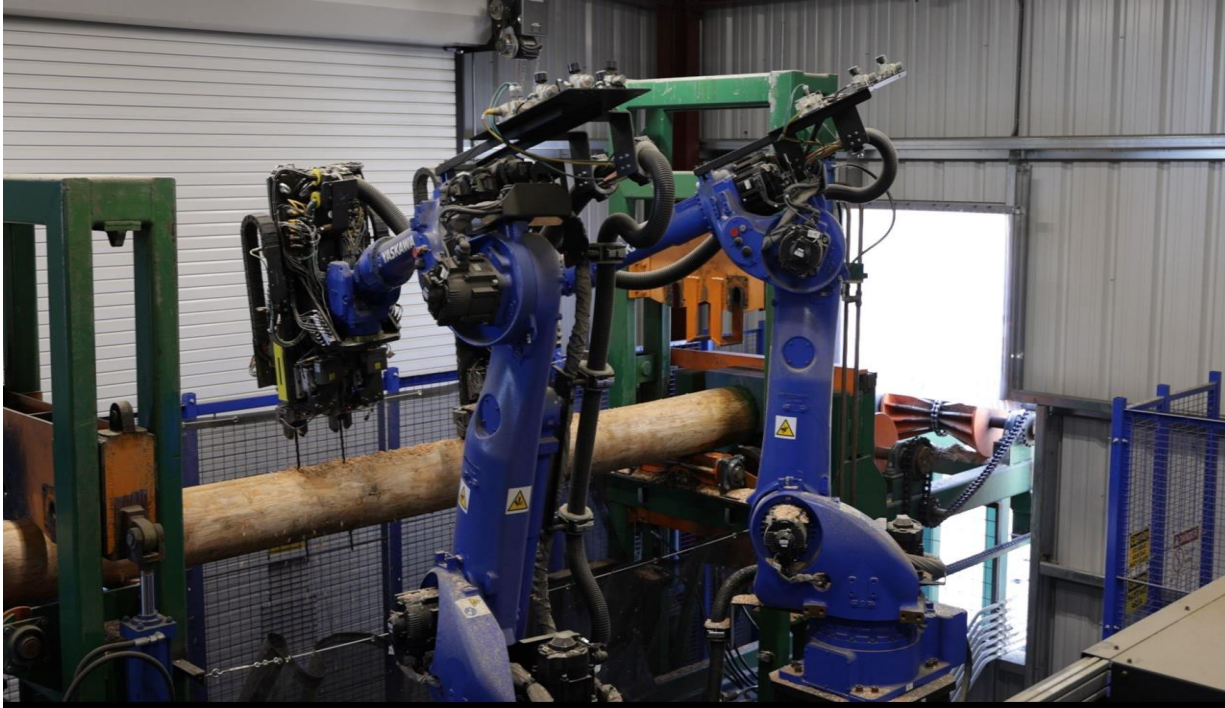
Robotic framing line, Eugene, Oregon
